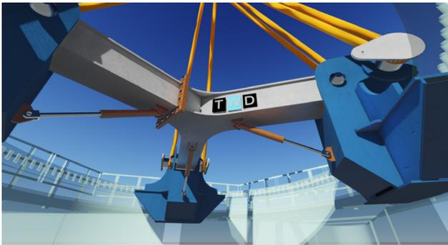
The Jacket Lifting Tool saves significant installation and operation time, since crew access or guides on the jacket are not needed during installation and lifting. Due to the specific shape of the clamping hooks the tool positions itself on the jacket's flange. With the rollers, the orientation of the tool is altered, while being monitored by cameras and sensors.
